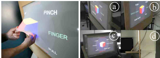
Figure 2: The prototype of an elastic, deformable display used in the study (left). The video recorded by the four cameras (right).
