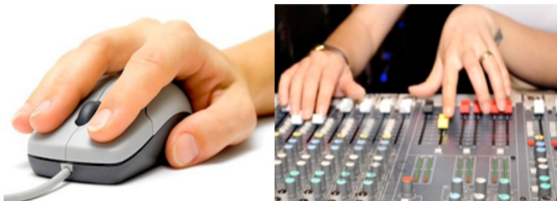
Figure 5: A classical example of a time multiplexed control (mouse) and a spatial multiplexed one (mixer). While with the former many parameters are modified sequentially in time with the use of one device, with the latter many parameters are modified at the same time through the use of many dedicated transducers for each parameter
